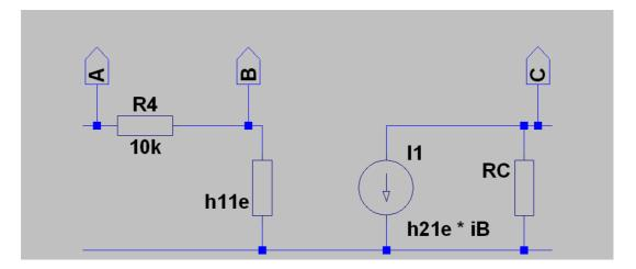
Please assume that  $h_{21e} = \beta$  and calculate the theoretical gain of the circuit. How does it compare to the result of measurements?
