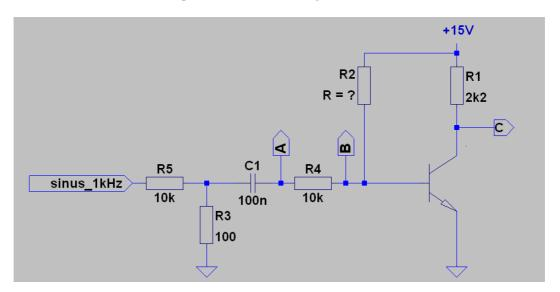
Please adjust the amplitude of the input sinusoidal signal so that the output AC voltage (oscilloscope in AC mode) in the point marked as C is about 2.5V. Please measure the AC voltages in points A and B using oscilloscope in AC mode.
