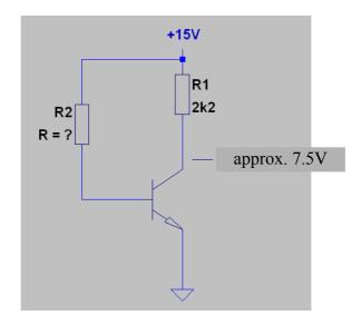
Calculate the value of R2 using the previously measured  $\beta = f(I_c)$  characteristic.
