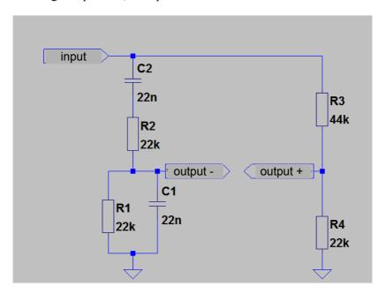
Please observe the changes of amplitude and phase of the signal on the output of the bridge (between points "output -" and "output +"). It will be necessary to use mathematical functions of the oscilloscope – the difference between two ground referenced channels. Please explain why it is necessary to use this kind of operation.
