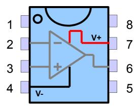
2. Symmetrical power supply  $\pm 15$ V used to power the amplifier during this lab can be obtained using the connections shown below (*Series* mode needs to be activated):
