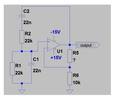
Please observe the output signal and measure its frequency. How does it correspond to the previously measured frequencies? Please explain the cause of output signal distortions
