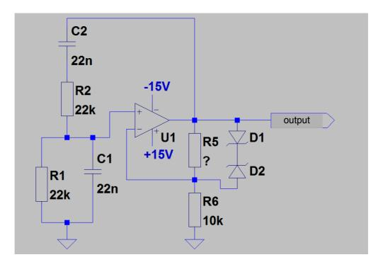
Please observe the output signal and measure its frequency. How does it correspond to the previously measured frequencies? Please explain how do the diodes influence the circuit behaviour
