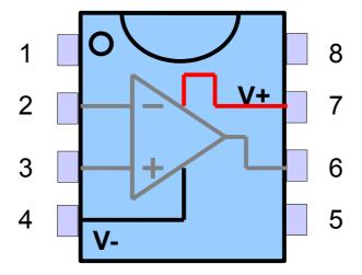
1. Symmetrical power supply  $\pm 15V$  used to power the amplifier during this lab can be obtained using the connections shown below (*Series* mode needs to be activated):
