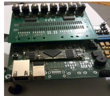
Figure 7. Board with FPGA and D/C converters
