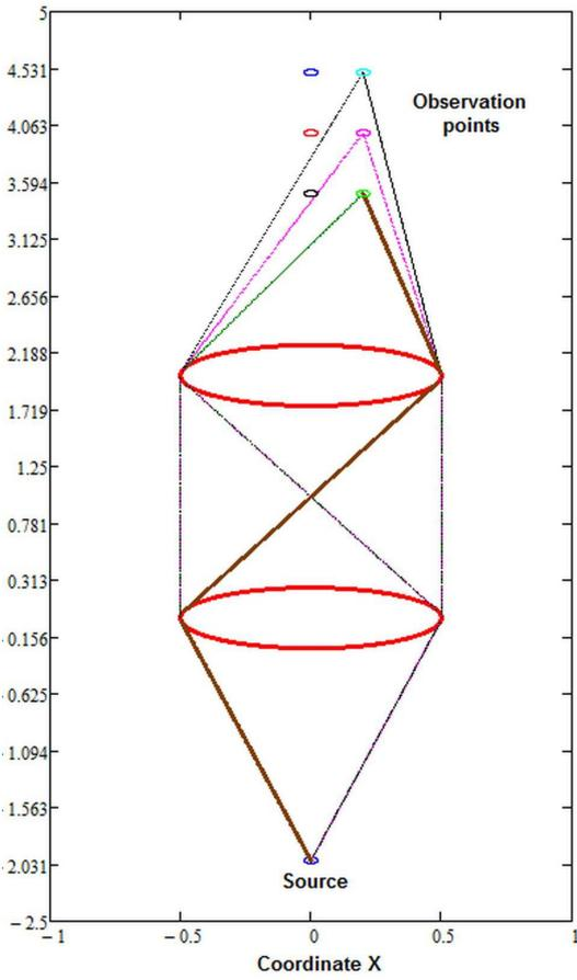
Fig. 2. Propagation scenario corresponding to the second numerical example. A Bold (brown color) ray is taken into consideration.
