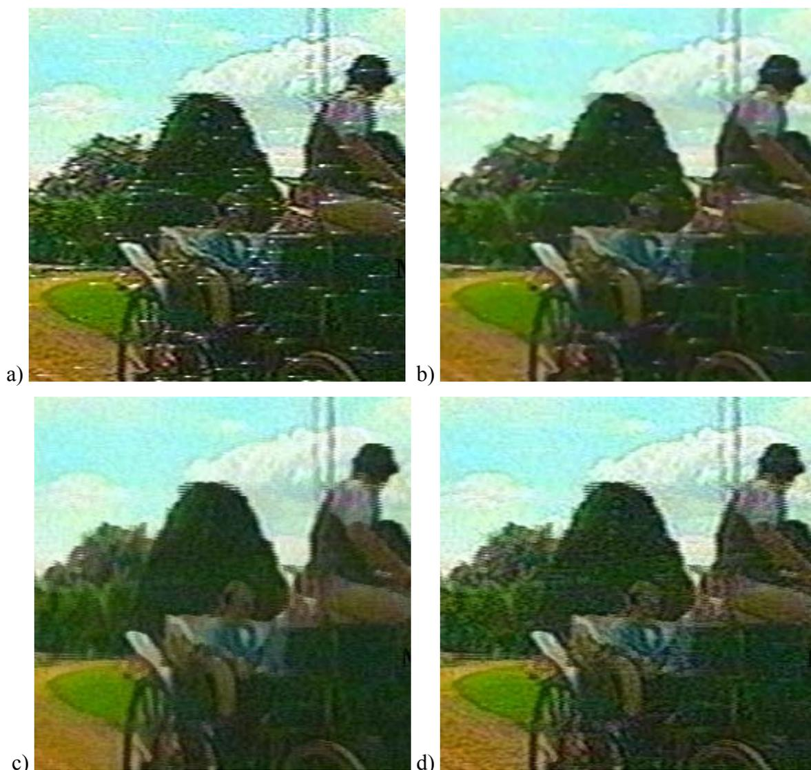
Figure 6.10. A selected frame from a television satellite receiver before and after processing, a) a corrupted frame with comet-like impulse noise, b) an output of two-dimensional recursive vector median filter with progress-wise window, c) an output of two-dimensional recursive vector median filter with interlace-wise window, d) and an output of three-dimensional recursive vector median with prediction error processing using interlace-wise window.
