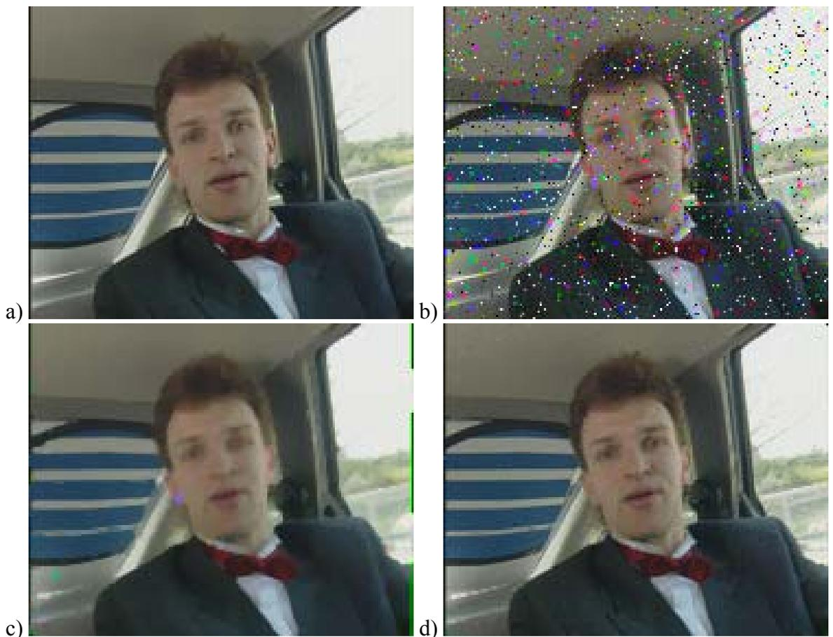
Figure 6.4. Selected frame of *Carphone* sequence: a) the original, b) corrupted with impulse noise ( $p = 5\%$ ), c) two-dimensional vector median filter RVMF output, d) recursive vector median filter with prediction error processing and motion-compensation RVMPCF output.
