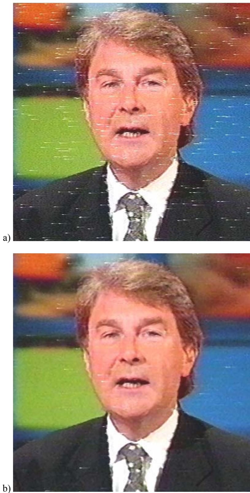
Figure 6.16a. A selected frame from a television satellite receiver before and after processing, corrupted frame with comet-like impulse noise (top), an output of two-dimensional recursive vector median filter by using of progress-wise window (bottom).
