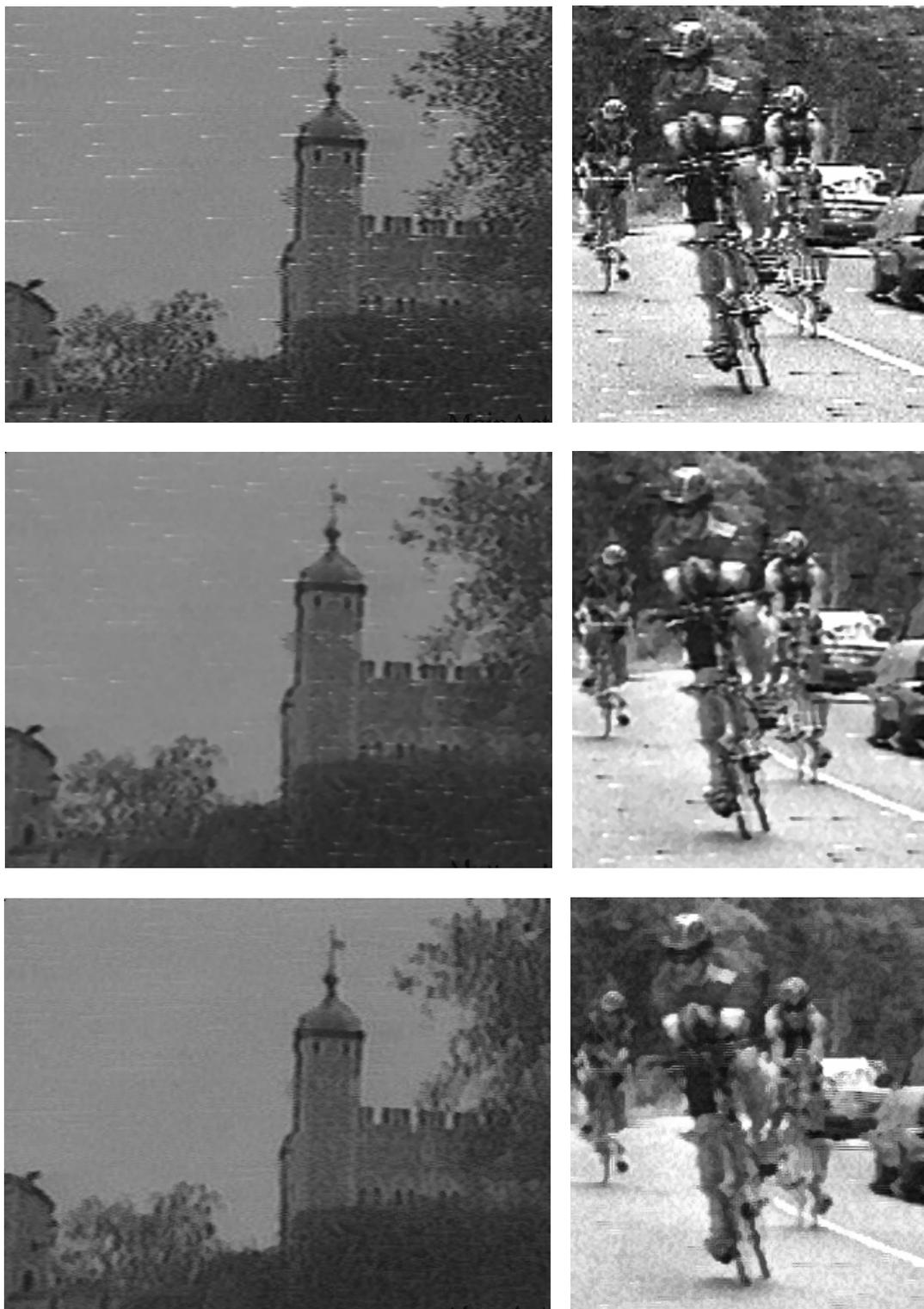
Figure 6.12. A selected frame from a television satellite receiver before and after processing: corrupted frame with comet-like impulse noise (up), an output of two-dimensional recursive vector median filter using progress-wise window (middle), and an output of three-dimensional recursive vector median with prediction error processing when an interlace-wise window is used (down).
