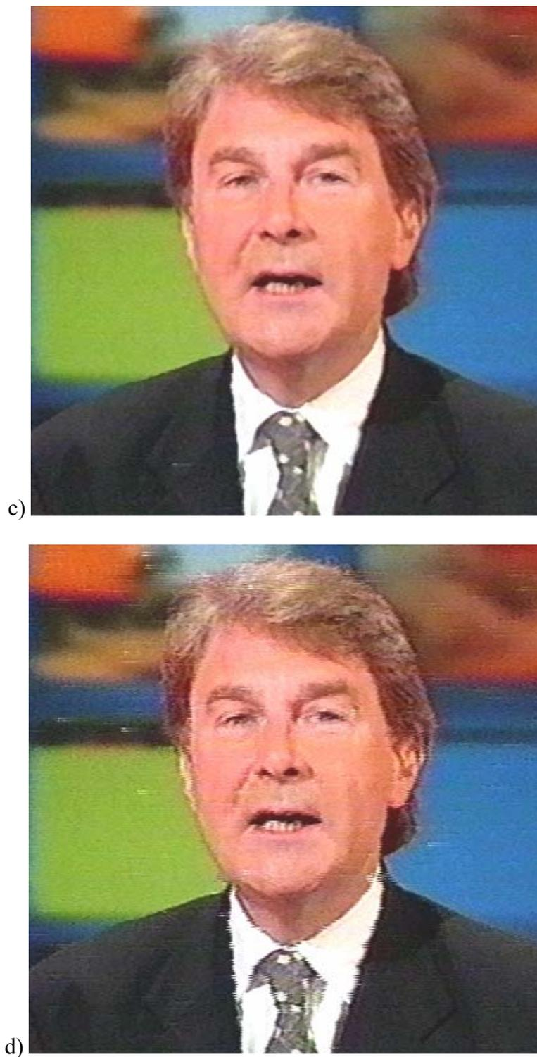
Figure 6.16b. A selected frame from a television satellite receiver before and after processing: an output of two-dimensional recursive vector median filter when an interlace-wise window is used (top), and an output of three-dimensional recursive vector median with prediction error processing when an interlace-wise window is used with adaptive threshold  $\alpha_E$  (bottom).
