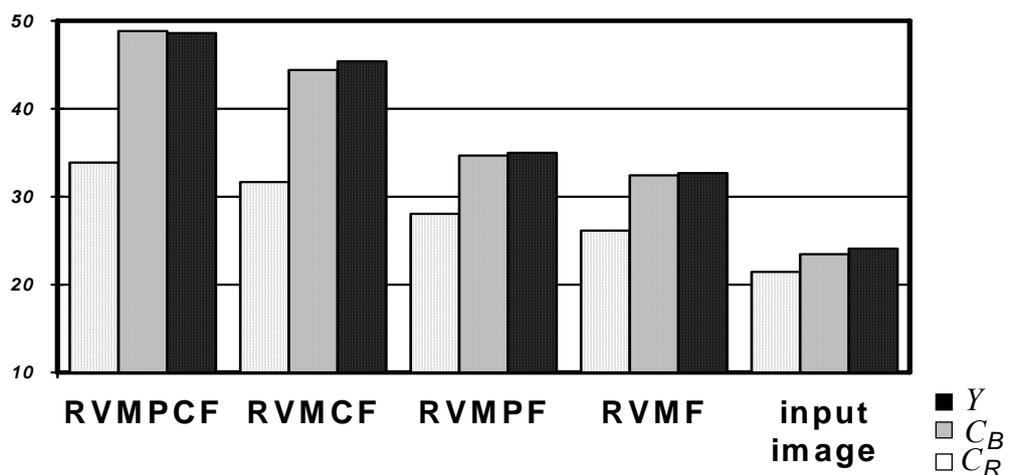
Figure 6.3. The output of vector recursive median filters in *PSNR* calculated for each color component  $Y$ ,  $C_B$ , and  $C_R$  for the fourth frame of the *Carphone* image sequences. Noise probability is  $p = 5\%$  of Type A, adaptive estimation of the parameter  $\alpha$  is applied.
