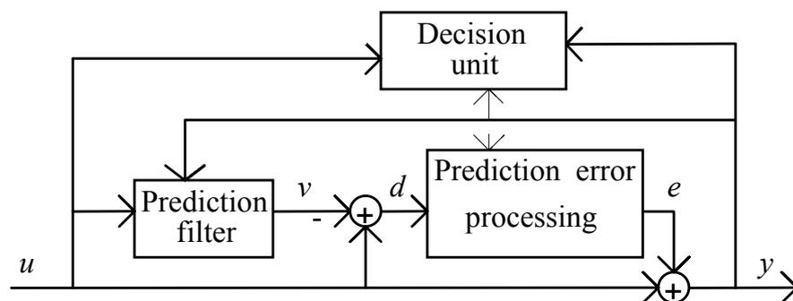
Figure 4.4. Basic structure of filter with prediction error processing.
