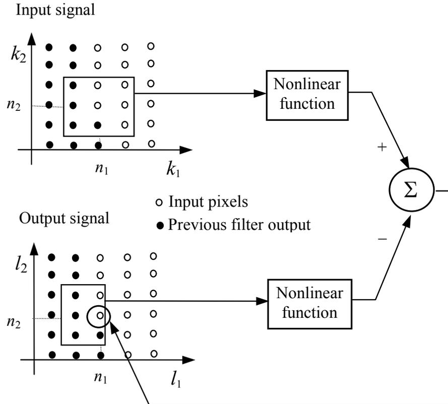
Figure 4.6. Example of the input and output masks for recursive filter.
