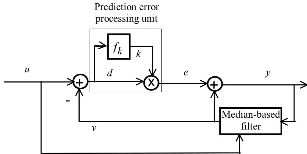
Figure 5.1. A structure of a filter with prediction error processing.
