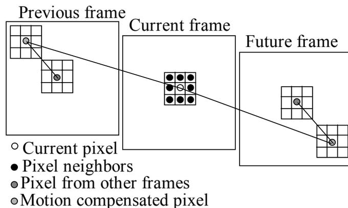
Figure 3.3. Support of a motion-compensated three-dimensional filter.
