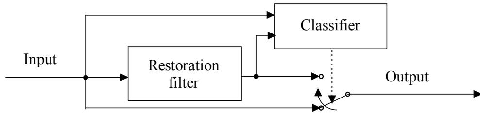
Figure 4.1. Basic structure of decision-based filter.
