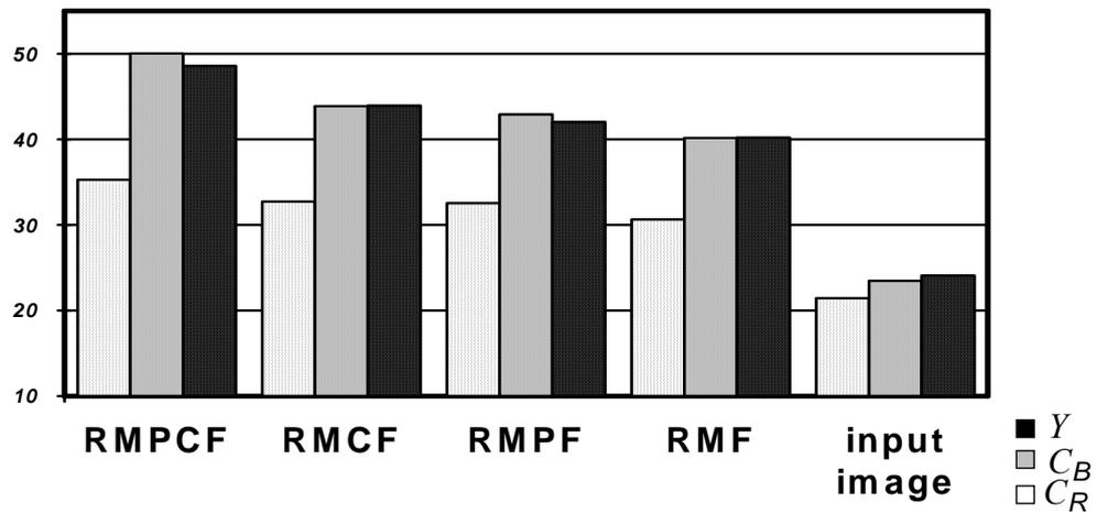
Figure 6.2. The output of component-wise recursive median filters in *PSNR* calculated for each color component  $Y$ ,  $C_B$ , and  $C_R$  for the fourth frame of the *Carphone* image sequences. Noise probability is  $p=5\%$  of Type A, adaptive estimation of the parameter  $\alpha$  is applied.
