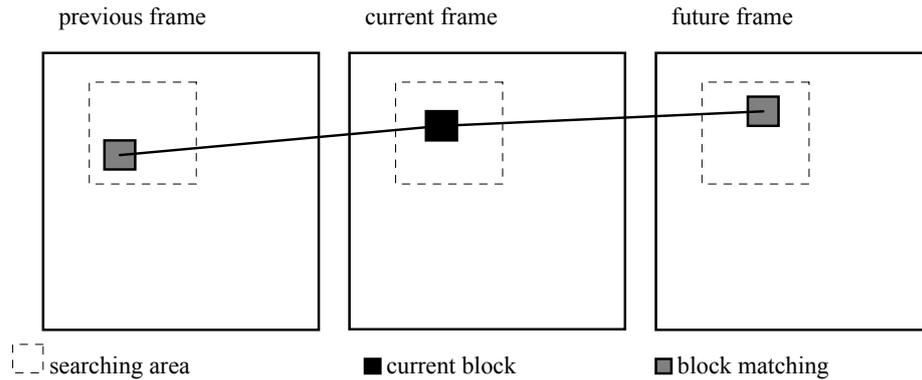
Figure 3.2. Principle of motion estimation.
