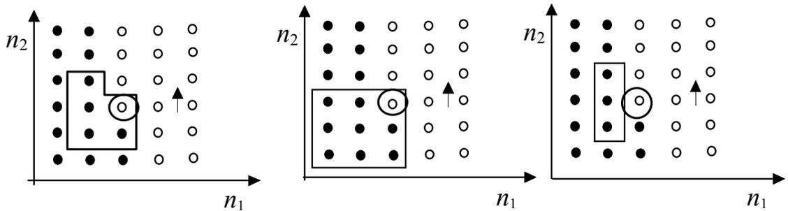
Figure 4.7. Different shapes of the output mask of recursive filter.
