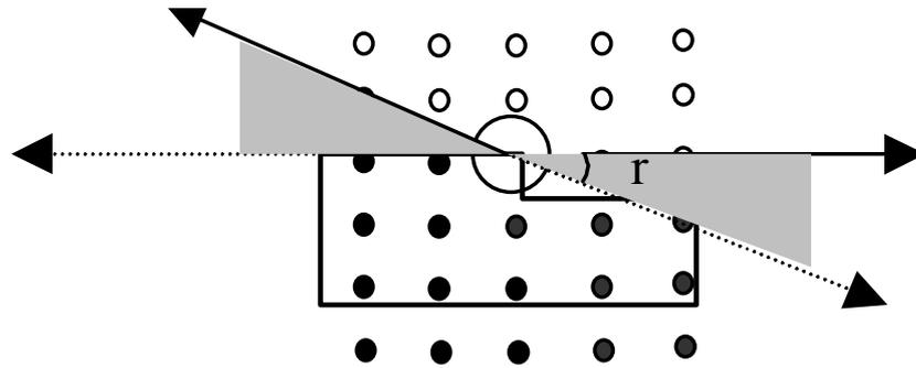
Figure 4.8. The rotation angle ( $r$ ) of the allowable direction of recursion.
