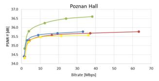
FIGURE 8. PSNR-Y RD-curves for PoznanHall sequence for encoding with original depth maps (red curve), with depth maps refined with the proposal (green), synthesis-based refinement (blue), and bilateral filter (yellow).
