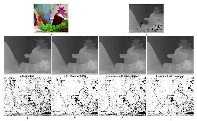
FIGURE 11. Comparison of depth maps for Teddy test images: (a) input image. Depth map: (b) ground-truth, (c) estimated, (d) refined with synthesis-based refinement, (d) bilateral filter (f) proposal. Bad pixels of depth map: (g) estimated, (h) refined with synthesis-based refinement, (i) bilateral filter, (j) proposal.
