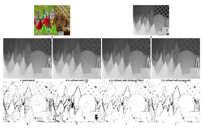
FIGURE 10. Comparison of depth maps for Cones test images: (a) input image. Depth map: (b) ground-truth, (c) estimated, (d) refined with synthesis-based refinement, (d) bilateral filter (f) proposal. Bad pixels of depth map: (g) estimated, (h) refined with synthesis-based refinement, (i) bilateral filter, (j) proposal.
