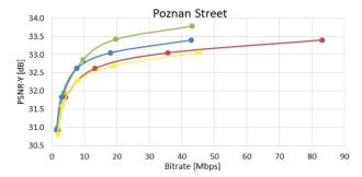
FIGURE 9. PSNR-Y RD-curves for PoznanStreet sequence for encoding with original depth maps (red curve), with depth maps refined with the proposal (green), synthesis-based refinement (blue), and bilateral filter (yellow).
