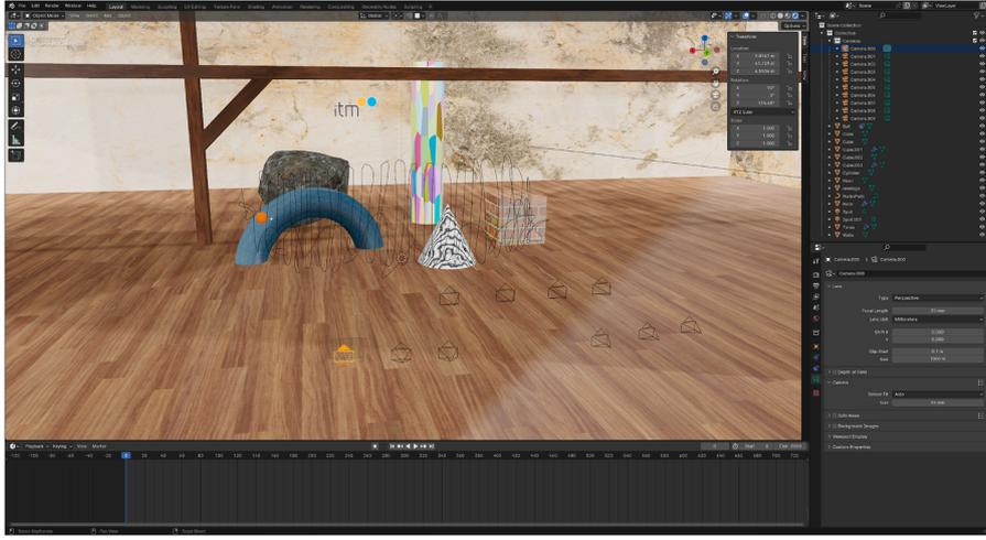
Fig. 2. The Blender project contains a test scene with 10 cameras, several static objects, and a moving calibration marker.
