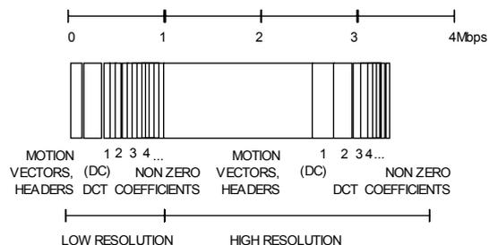
Fig. 4. Bitstream structure for the progressive test sequence *Flower Garden* with total bitrate 3.31 Mbps
