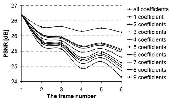
Fig. 9. Decreasing signal-to-noise ratio according to drift for various numbers of DCT coefficients per block transmitted in the enhancement layer to the decoder. Test sequence *Funfair* with an average bitrate 0.5 Mbps and without B-frames.
