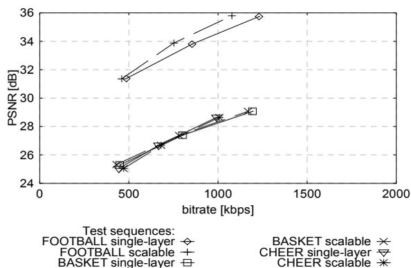
Fig. 5. Coding efficiency (luminance PSNR versus bitrate) for the two-loop structures based on H.263 baseline coder (temporal subsampling factor = 2, image resolution – CIF, 30 fps).
