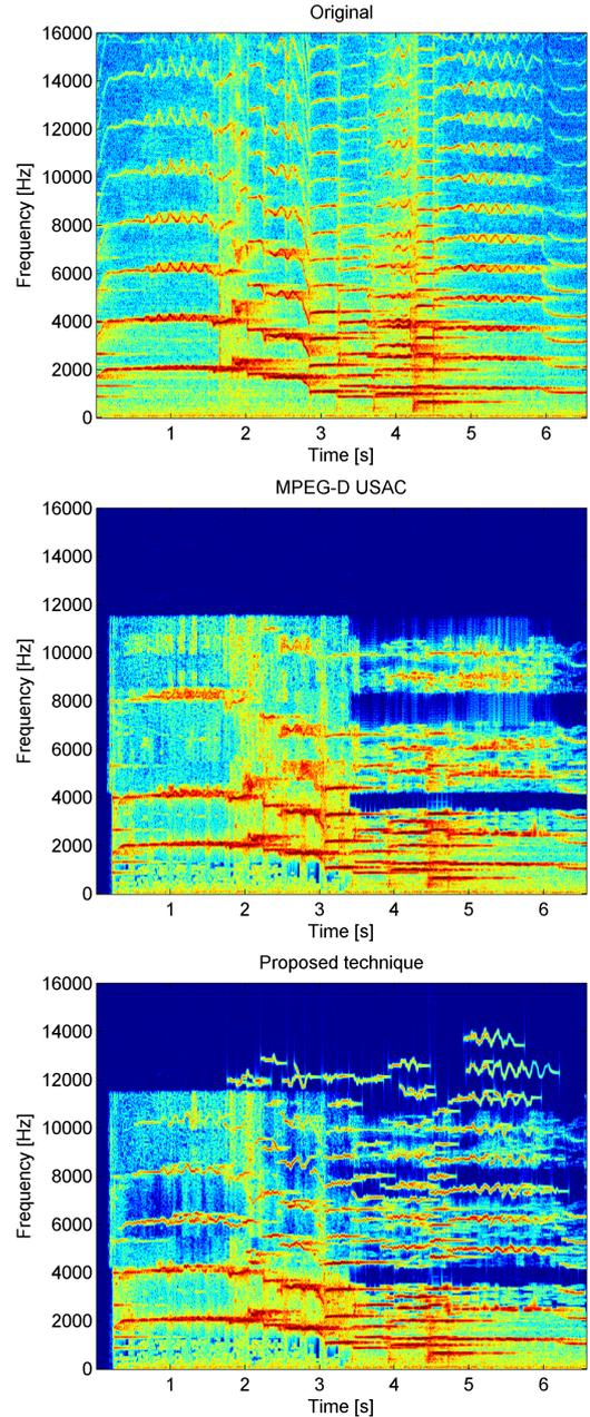
**Fig. 3.** Example spectrograms for signal violin2 and target bit-rate of 16 kb/s, from the top: input signal, full reconstructed signal in the decoder (MPEG-D USAC), full reconstructed signal in the decoder (proposed technique).
