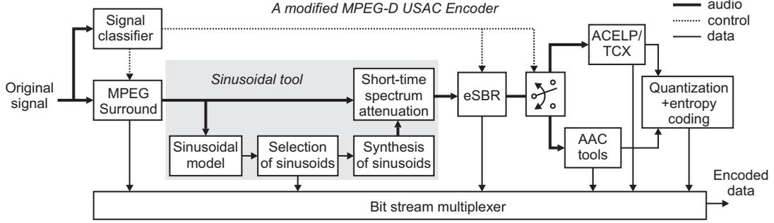
Fig. 1. The modified MPEG-D USAC encoder with additional blocks related to the proposed sinusoidal tool.
