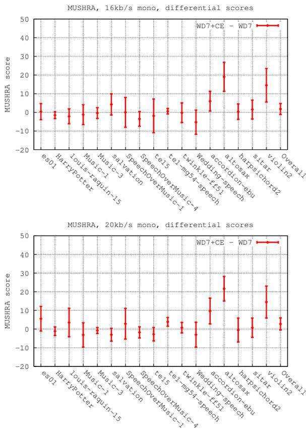
**Fig. 4.** Subjective test results at 16 kb/s (top) and 20 kb/s (bottom) - differential scores (WD7-CE vs WD7). The 95 % confidence intervals (8 listeners) are plotted.
