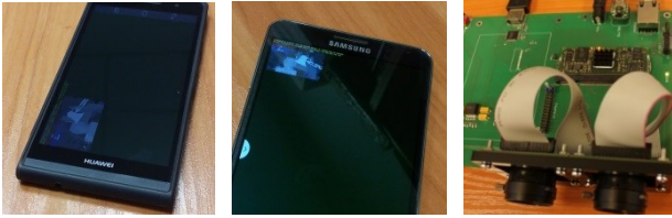
Figure 3. The proposed disparity estimation algorithm implemented on Android mobile devices (Huawei Ascend P6, Samsung Galaxy Note 3) and on the processing board developed by the authors equipped with Xilinx Artix-7 FPGA
