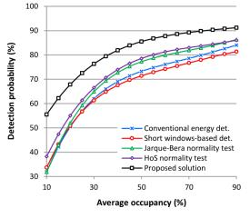
**FIGURE 5.**  $P_d(\tau)$  function for the observation window size of N = 1024 samples, type I error probability  $P_f = 10\%$ , and SNR = -6dB.
