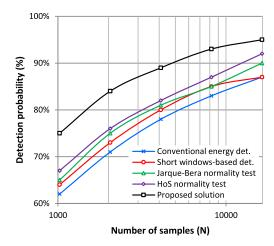
**FIGURE 9.**  $P_d(N)$  function for average transmitter activity  $\tau = 30\%$ , type I error probability  $P_f = 10\%$ , and SNR = -6dB.
