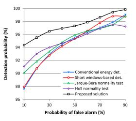
**FIGURE 7.**  $P_d(P_f)$  function for the observation window size of N = 16384 samples, average transmitter activity  $\tau = 30\%$ , and SNR = -6dB.
