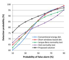
**FIGURE 4.**  $P_d(P_f)$  function for the observation window size of N = 1024 samples, average transmitter activity  $\tau = 30\%$ , and SNR = -6dB.
