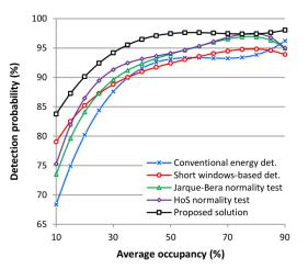
**FIGURE 8.**  $P_d(\tau)$  function for the observation window size of N = 16384 samples, type I error probability  $P_f = 10\%$ , and SNR = -6dB.
