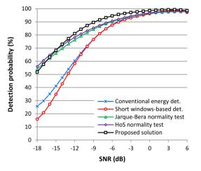
**FIGURE 6.**  $P_d$  (SNR) function for the observation window size of N = 16384 samples, average transmitter activity  $\tau = 30\%$ , and type I error probability  $P_f = 10\%$ .
