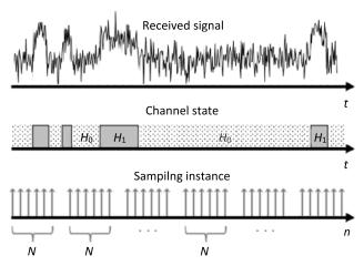
FIGURE 1. Illustration of discontinuous transmission with marked channel states and detector sampling periods.
