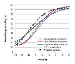
**FIGURE 3.**  $P_d$  (SNR) function for the observation window size of N = 1024 samples, average transmitter activity  $\tau = 30\%$ , and type I error probability  $P_f = 10\%$ .
