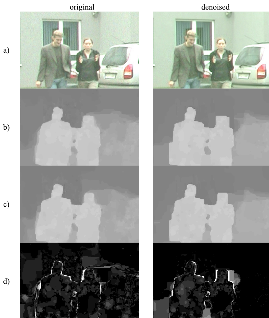
Fig. 9. Exemplary results of proposed technique: original (left) and denoised (right). a) image b,c) depth maps for two consecutive frames d) difference between depth maps.
