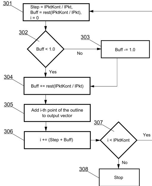
**Fig. 3.** Evenly Distributed Points - algorithm block diagram.
