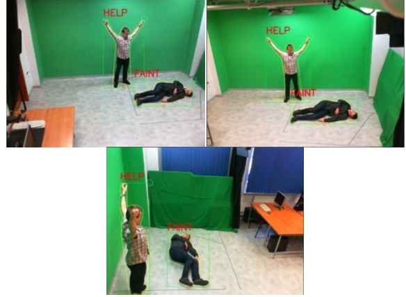
Figure 7: Results of detection two human activity ("Calling for Help" and "Faint") in one scene for 3 cameras.
