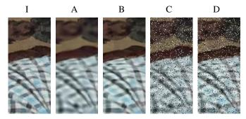
Fig. 5. I: Fragment of input video (sequence Frog [83]), A: fragment I compressed by VVC [112] with QP = 43, B: the same fragment of the synthesized view, C: fragment A with heavy salt-and-pepper impulse noise, D: fragment B with heavy salt-and-pepper impulse noise.
