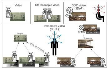
Fig. 1. An overview of the visual systems. Immersive video (bottom) utilizes virtual view synthesis performed using several input views and corresponding depth maps to provide a possibility of six-degrees-of-freedom movement for a viewer. 360° video (top right) enables only the change of orientation of viewing.
