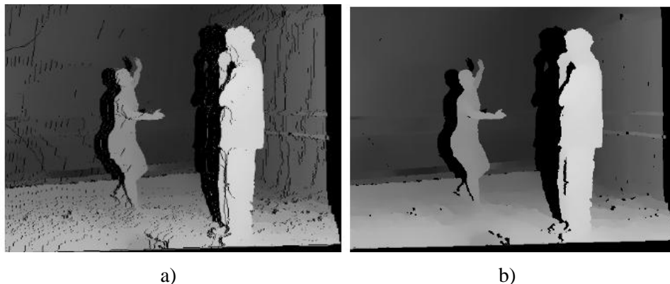
Figure 3. Depth map of synthesized view: a) before and b) after median filtering. Brighter points are closer. Black regions have unknown depth.
