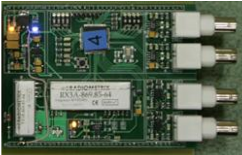
Figure 2. Wireless synchronization module.
