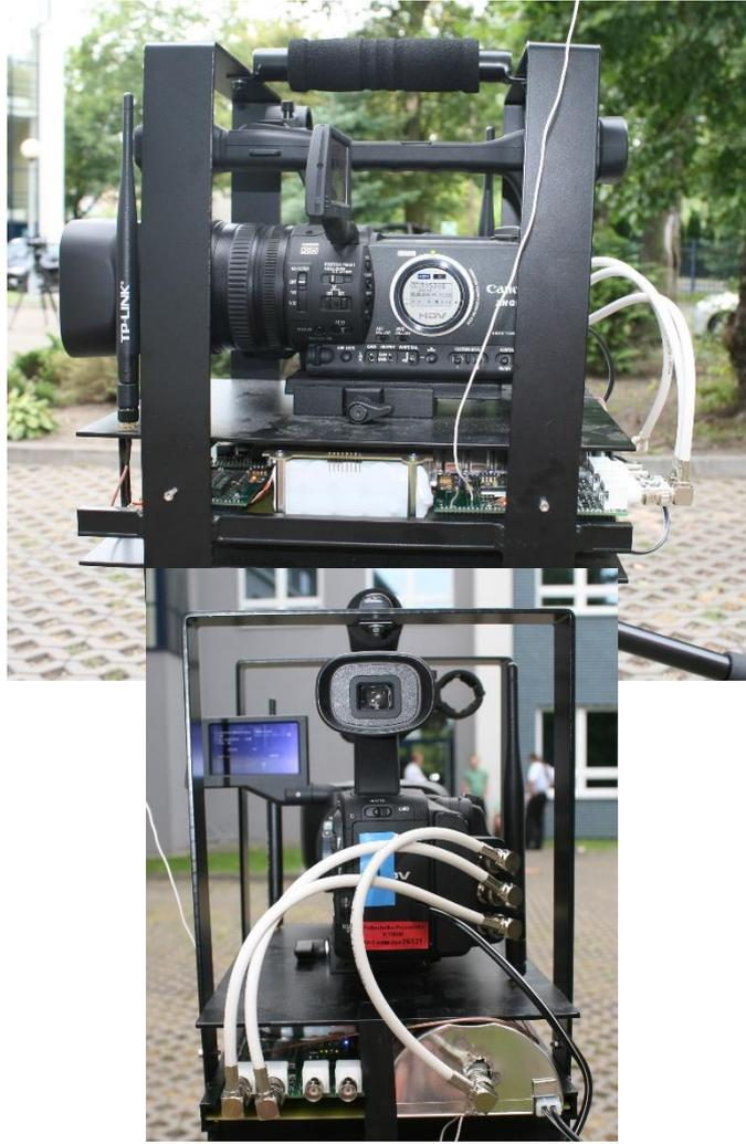
Figure 1. Wireless mobile camera module (side and rear views).
