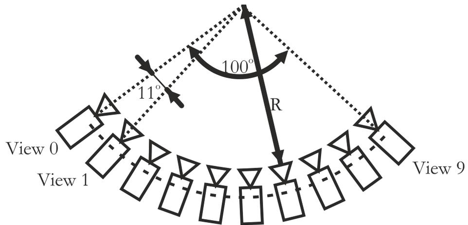
Figure 3. Circular camera setup used in the experiments reported in this document.
