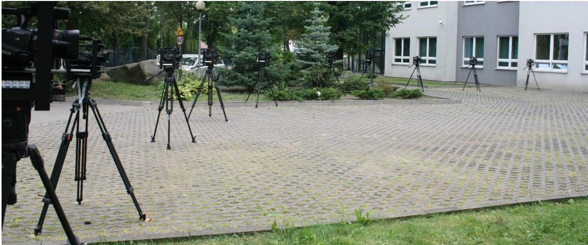
Figure 4. Multi-camera setup used in production of “Poznan Team” test sequence.
