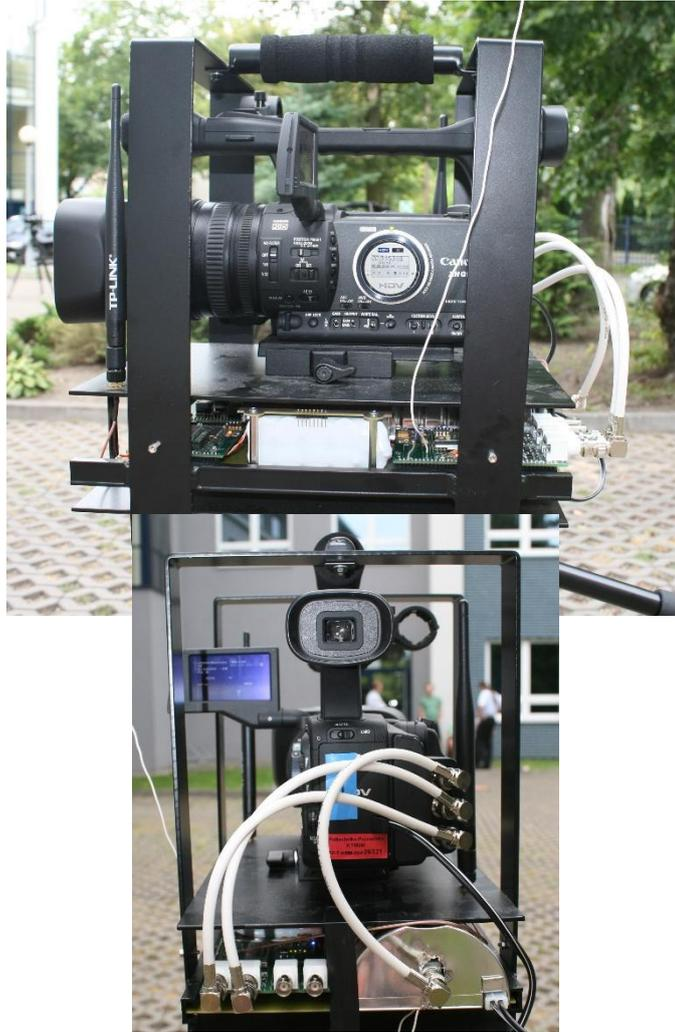
Figure 1. Wireless mobile camera module (side and rear views).
