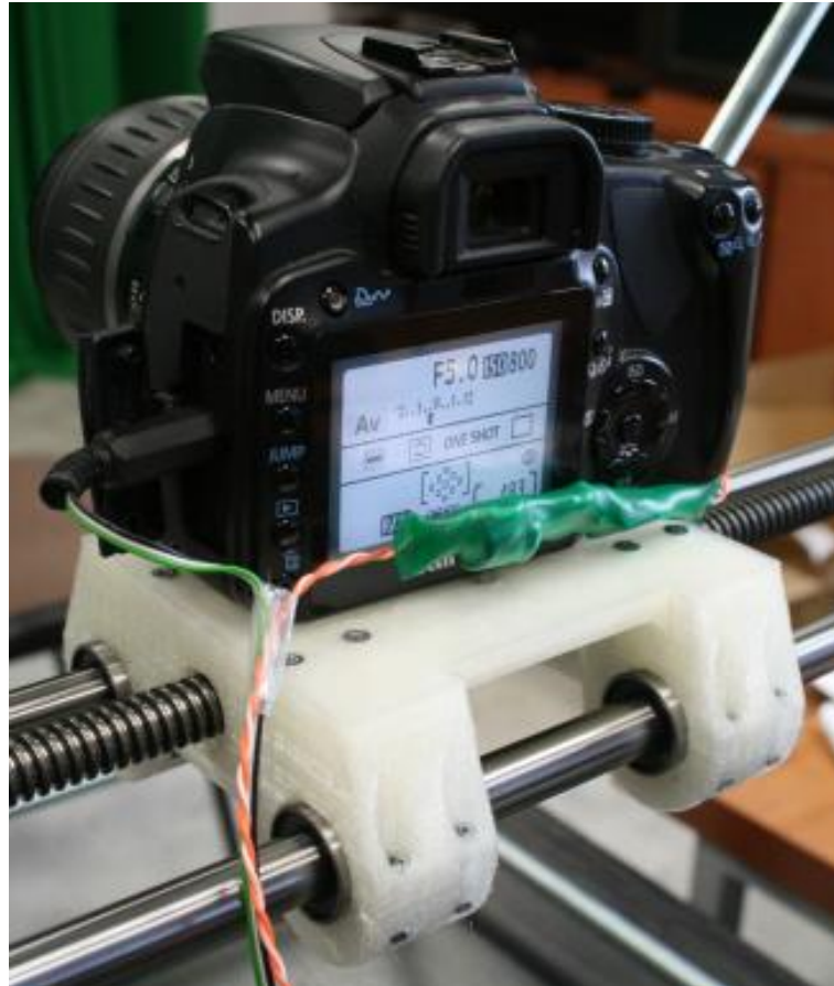
Figure 5. The camera fitted on the carriage together with automatic release and external power circuit.
