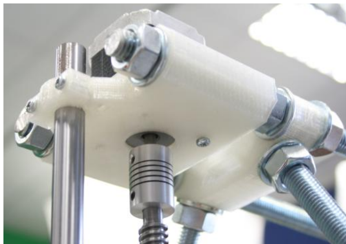
Figure 4. Vertical drive motor fitting.
