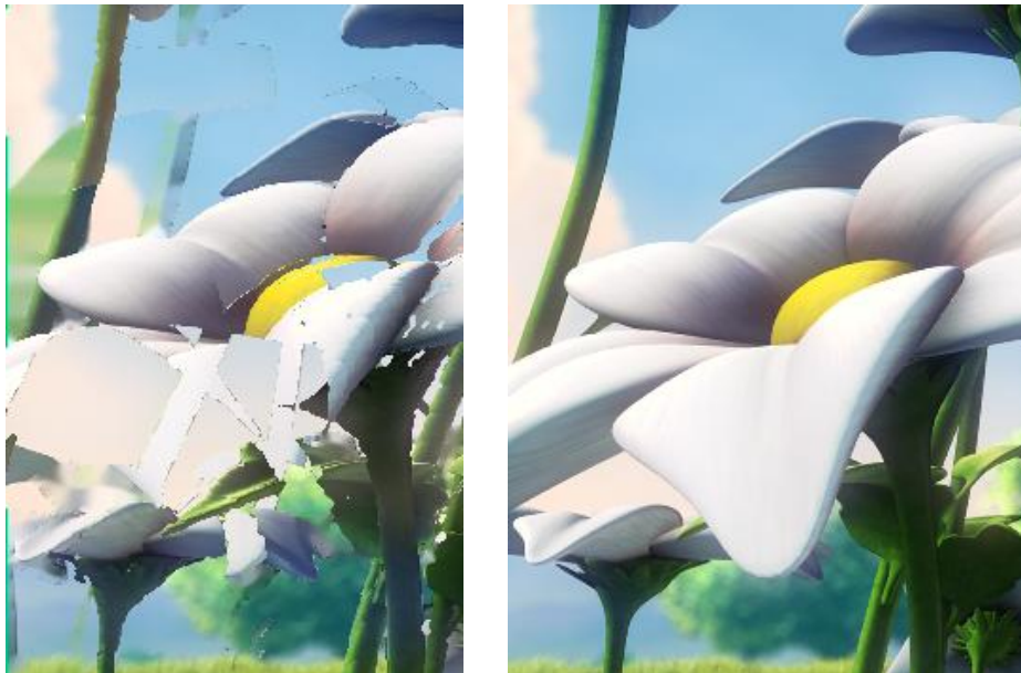
Figure 4. Example of wrongly synthesized views: synthesized virtual view (on the left) and the real one (on the right).
