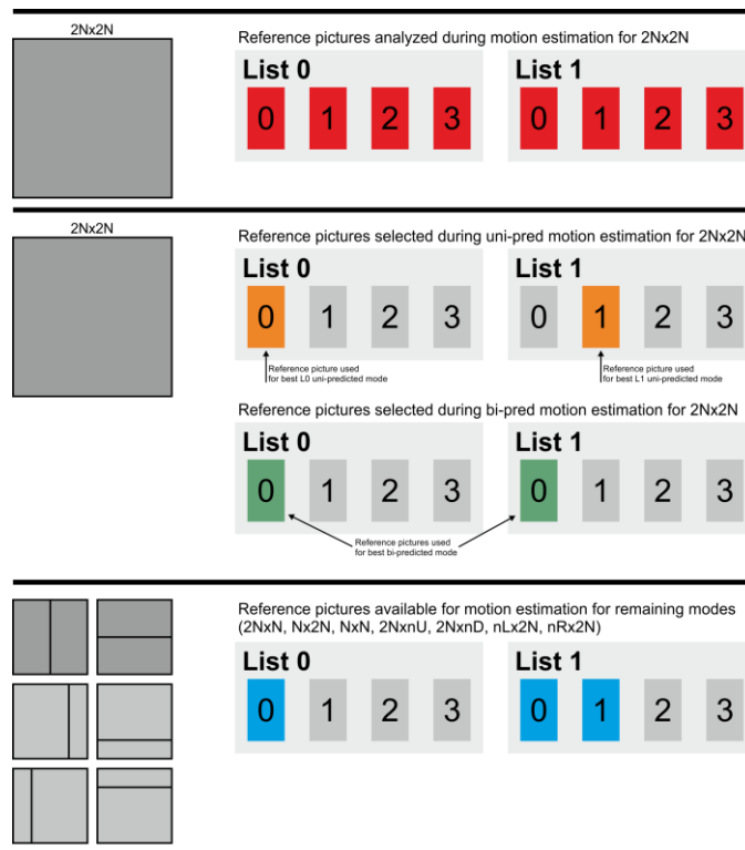
Fig. 1. Idea of reported method for fast reference picture selection. PUs of smaller size that 2N \times 2N considers only reference pictures that was considered the best for 2N \times 2N PU.
