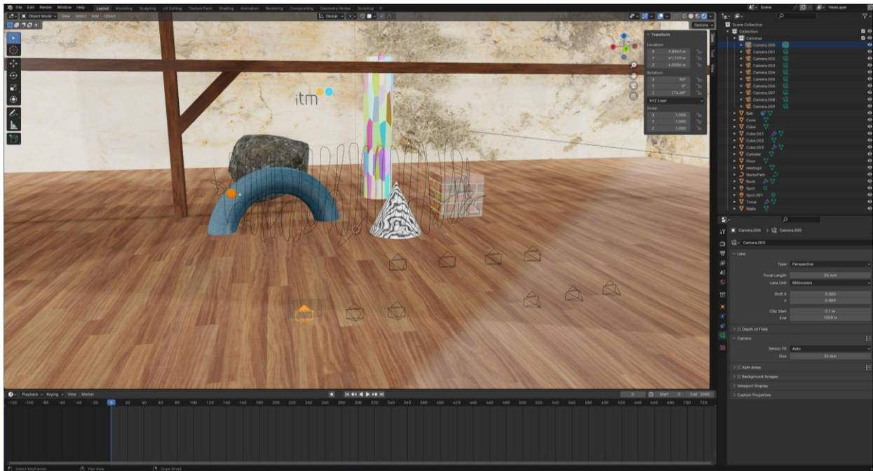
Figure 2. The Blender project contains a test scene with 10 cameras, several static objects, and a moving calibration marker.
