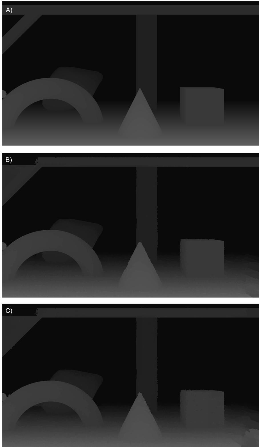
**Figure 4. Depth maps for view 6: A) rendered by Blender, B) estimated using exact camera parameters, C) estimated using calibrated camera parameters. The contrast of images was increased to highlight differences. Note that the quality of B is worse than for A because of imperfection of a depth estimation algorithm which cannot perfectly estimate depth for some parts of the scene (especially for areas acquired by a single camera (e.g., left top part of the view)).**
