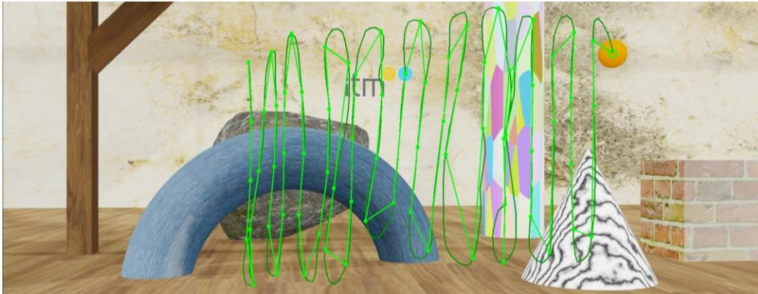
**Figure 3. Tracked marker. Yellow lines: the predicted path of a marker; green lines: the actual path measured by the marker tracker algorithm; blue rectangle: area in which the marker is being searched for;**
