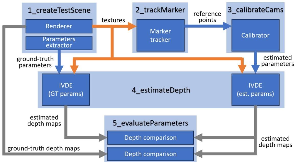
Figure 1. The general scheme of the ECPC software.
