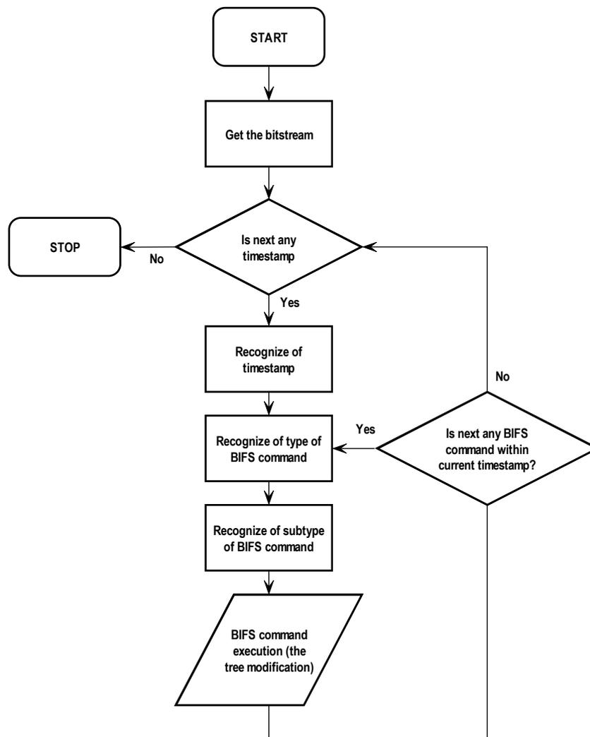
Fig.4. The algorithm of binary format decoder processing.
