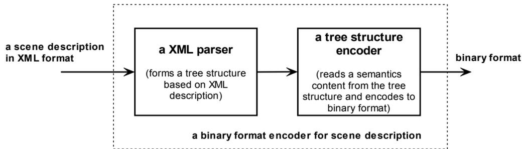
Fig.2. The block diagram of scene description encoder.
