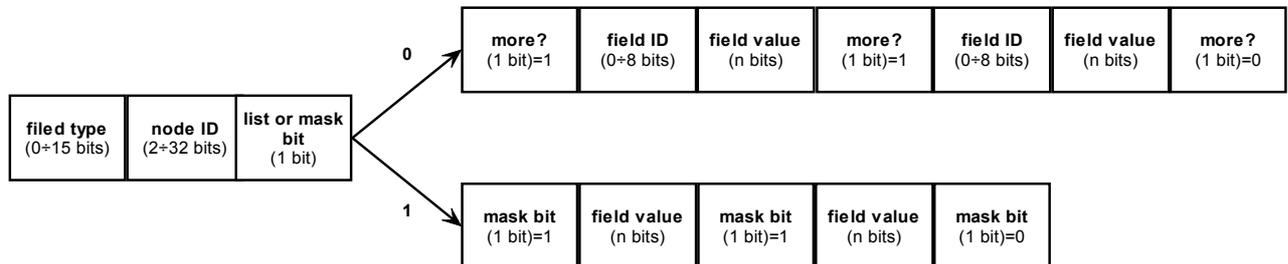
Fig.3. The example of the node encoding as a vector or a list.
