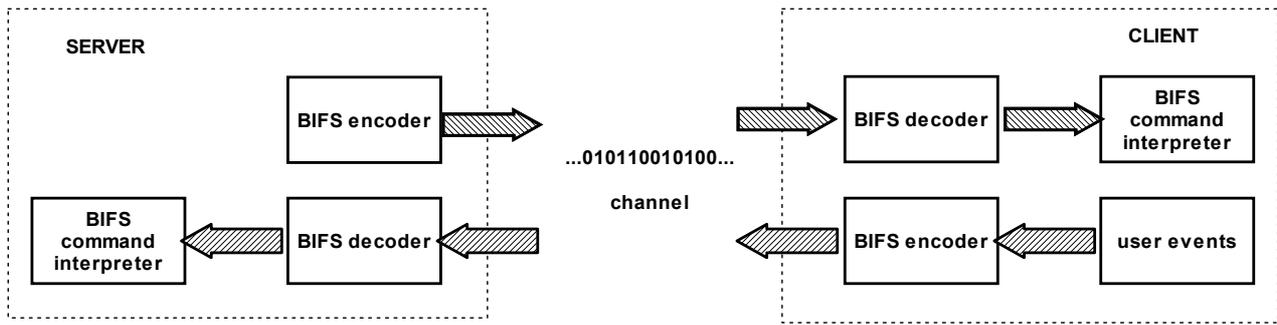
Fig.1. MPEG-4 client-server model and location of the BIFS encoder/decoder in the MPEG-4 system.
