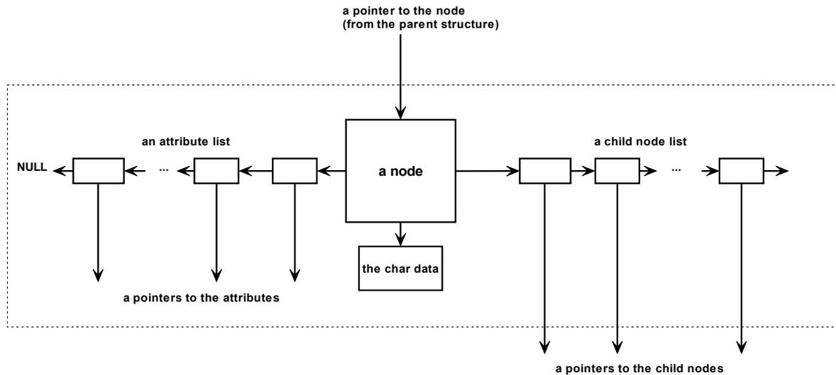
**Fig.5.** A scheme of the node in a memory allocated by the XML parser. The pointers to the nodes have a communication role between nodes in the tree.
