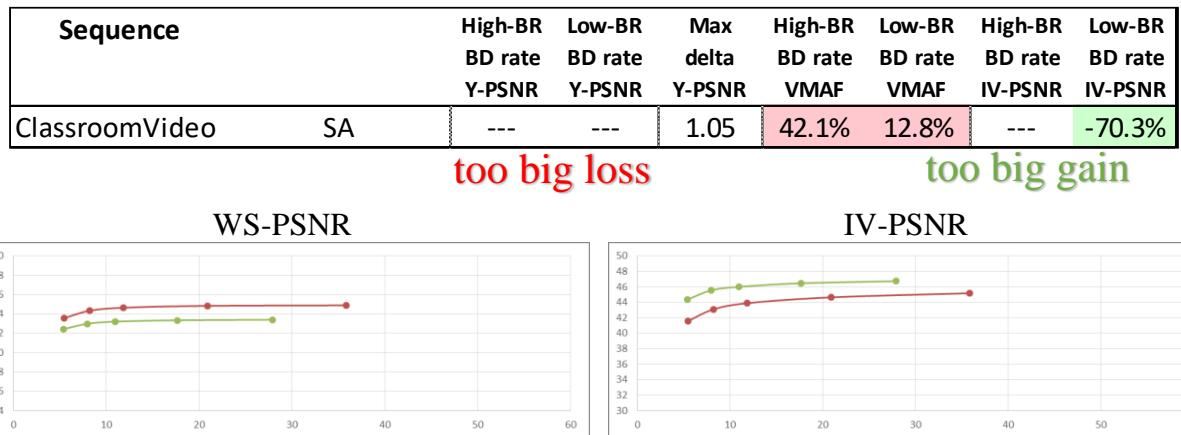
Fig. 5. WS-PSNR vs. IV-PSNR for SA (QP1 – QP5); red curve – anchor, green curve – proposed.
