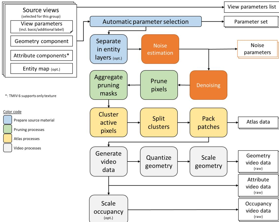
Fig. 1. TMIV encoder with proposed noise modelling.
