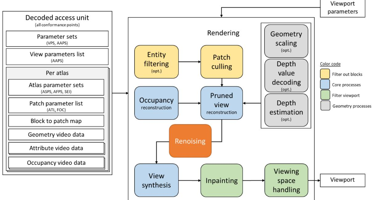
Fig. 2. TMIV decoder with proposed noise modelling.
