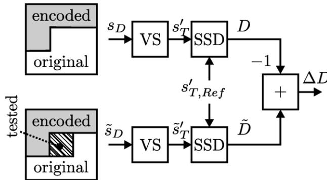
**Figure 28: Definition of the SVDC related to the distorted depth data of the block  $B$  depicted by the hatched area in the bottom branch; VS denotes the view synthesis step and SSD stands for sum of squared differences.**
