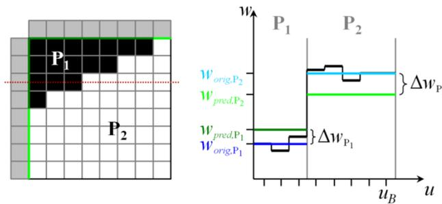
**Figure 20: CPVs of block partitions: CPV prediction from adjacent samples of neighbouring blocks (left) and cross section of block (right), showing relation between different CPV types.**
