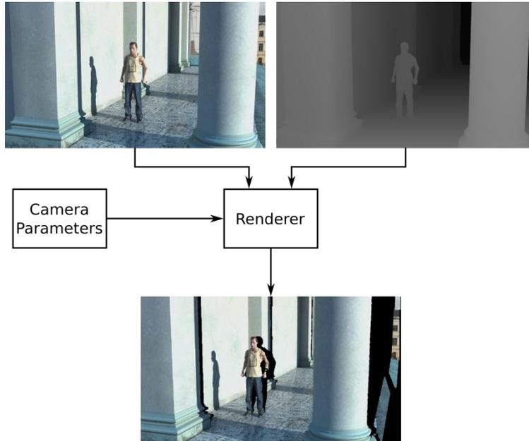
**Figure 31: Rendering from a left camera position to a right camera position using depth maps.**
