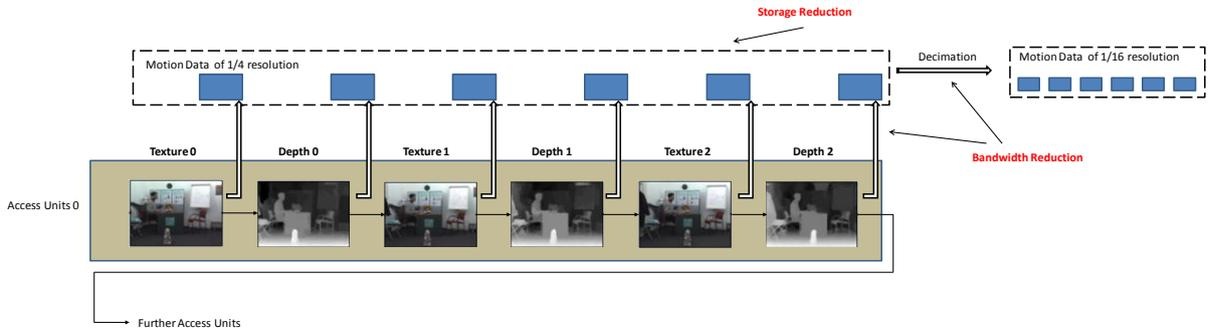
**Figure 27: Progressive motion compression for motion data buffer reduction.**
