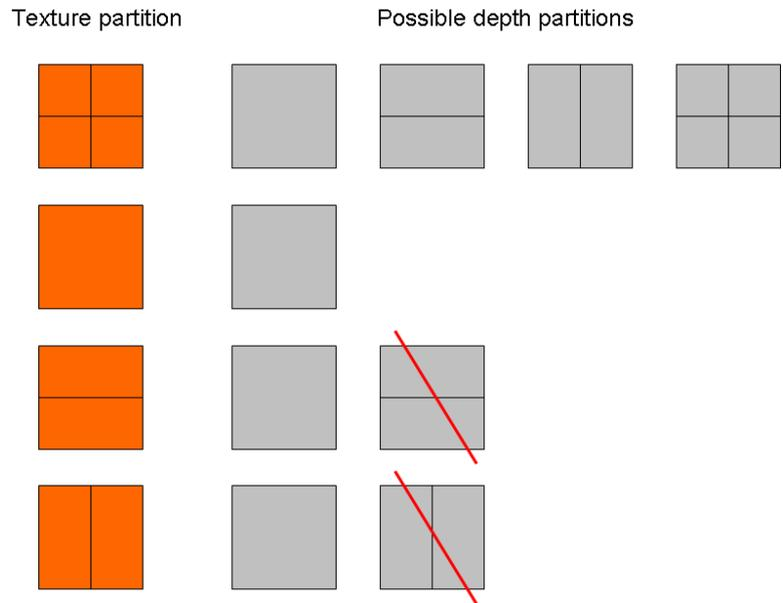
Figure 26: Texture partitions and corresponding possible depth partitions
