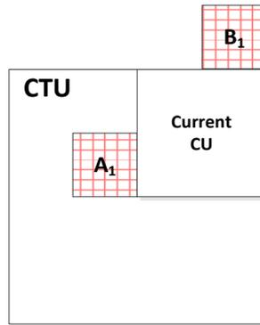
**Figure 7: Example: For the derivation of the disparity from DV-MCP neighbouring blocks of the current CU, above block B1 is not used, since it is not located within the current CTU.**
