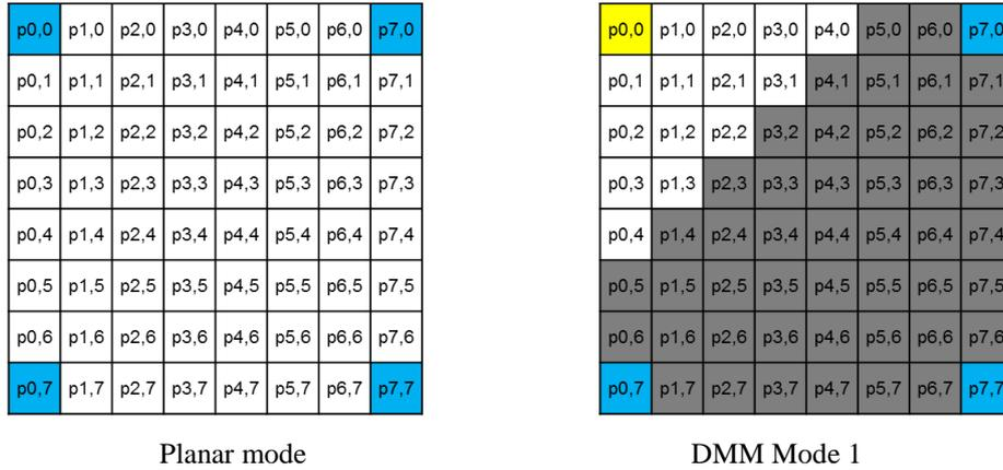
**Figure 23: Selection of samples for calculating the predicted depth value in SDC (Planar mode, DMM Mode 1)**
