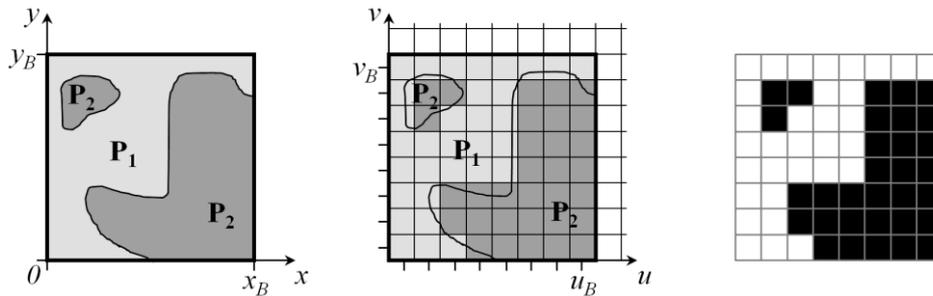
**Figure 19: Contour partition of a block: continuous (left) and discrete signal space (middle) with corresponding partition pattern (right).**
