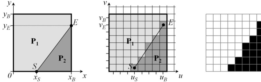
**Figure 18: Wedgelet partition of a block: continuous (left) and discrete signal space (middle) with corresponding partition pattern (right).**
