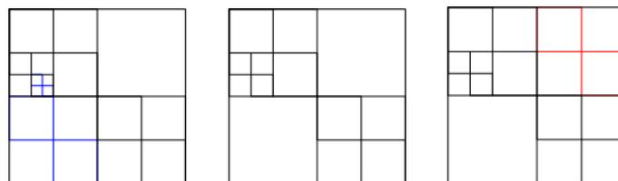
**Figure 30: Example of a CTB QT partitioning for the texture (left), allowed collocated depth CTB QT partitioning (centre), and disallowed collocated depth CTB QT partitioning (right).**
