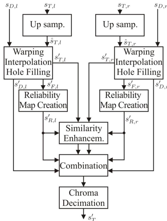
Figure 33: Processing steps of the view synthesis approach.
