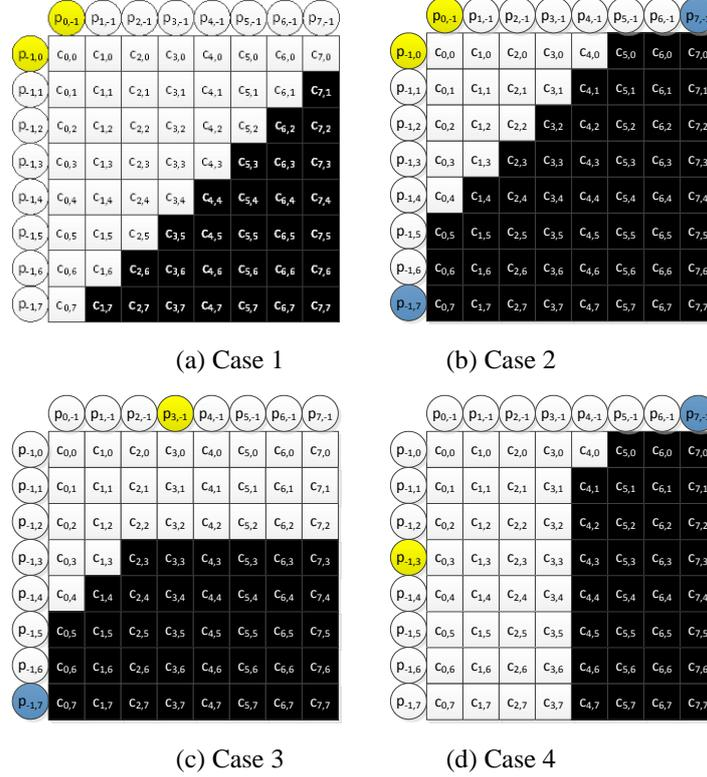
**Figure 21: Selection of reference samples for difference partition pattern cases.**
