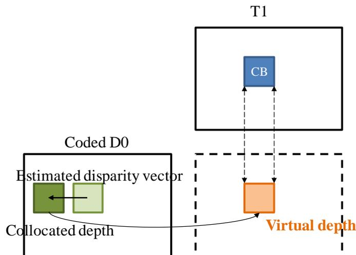
**Figure 8: Retrieval of the virtual depth block.**
