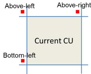
**Figure 25: Derivation of a disparity vector from three (red) neighboring reconstructed depth samples**
