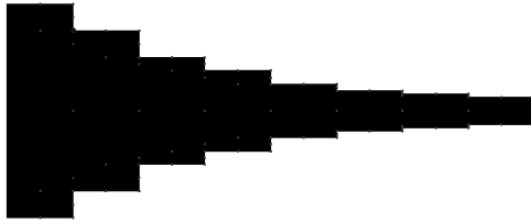
Fig. 3 Plan view of eight-section Ni - BaTiO 3 - Ni attenuation layer
