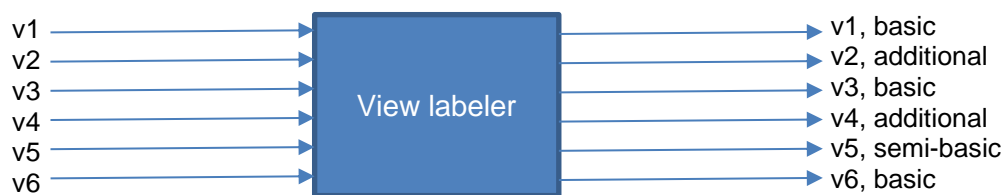
Figure 7: View selection behavior of the view labeler when semi-basic and additional views are enabled
