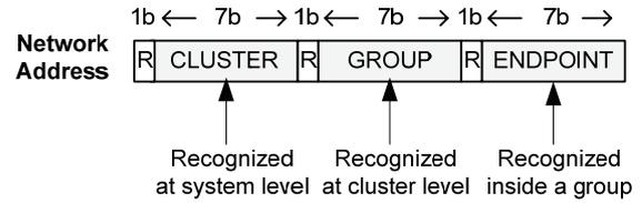
**Figure 5. Fields in a network address**
