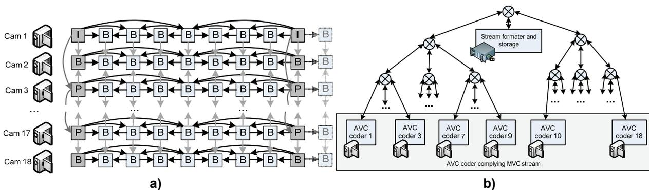
Figure 8. The MVC coding scheme (a) and the assessed model of the MVC coder (b)
