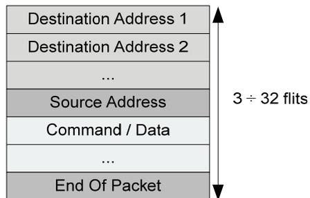
**Figure 6. The NoMC packet format**
