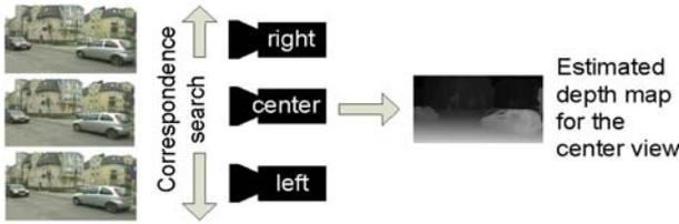
Figure 1. The scheme of considered 3-view depth estimation.
