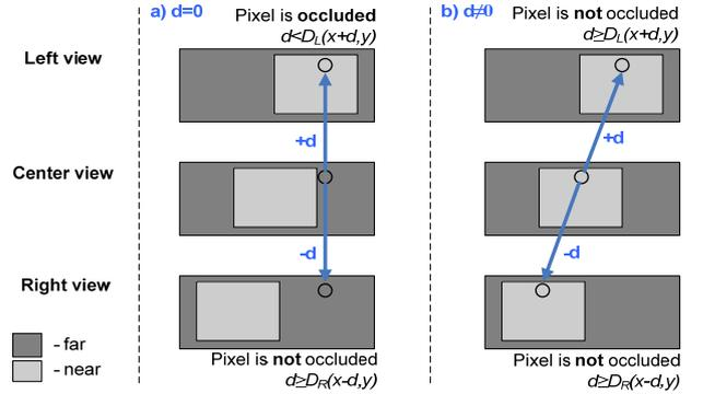
Figure 2. The correspondence of given pixel in the center view to the pixels in the neighboring views and proposed deduction of the occlusion – a) for far background objects and b) close foreground objects.
