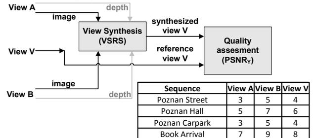
Figure 4. Depth map assesment procedure and view assignment for the test sequences.
