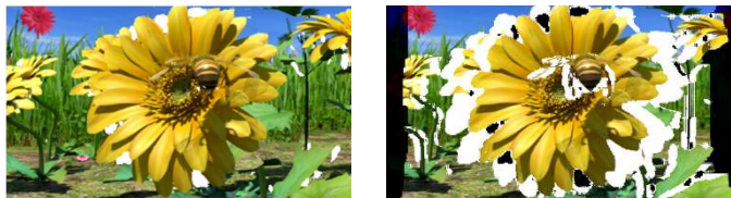
Figure 2. Occlusions in exemplary virtual view (white areas): left – non-synthesized regions (from any camera), right – partially synthesized regions (only from one camera).
