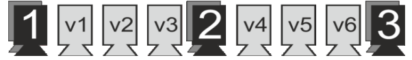
Fig. 3. The arrangement of the views in quality evaluation: the coded views are marked in black, while the synthesized virtual ("v") views are marked in gray.
