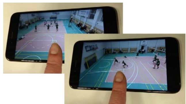
Fig. 6. Virtual navigation around the volleyball playfield controlled by motion of finger on a touchscreen of a smartphone.
