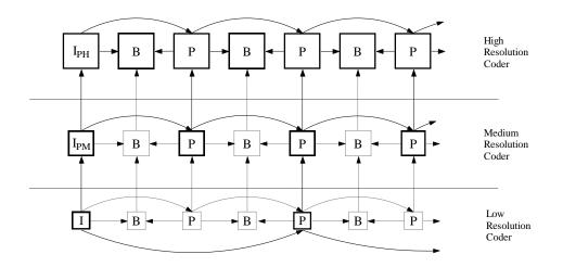
Fig.3. Exemplary structure of the video sequence.
