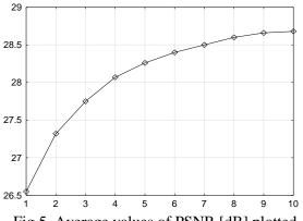
Fig.5. Average values of PSNR [dB] plotted versus the number of nonzero DCT coefficients allocated. Results for the *Cheer* test sequence, the high-resolution bitstream (MPEG-2 GOP=12, 2.35Mbps).
