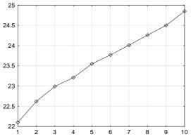
Fig. 4. Average values of PSNR [dB] plotted versus the number of nonzero DCT coefficients allocated. Results for the *Cheer* test sequence, the high-resolution bitstream
