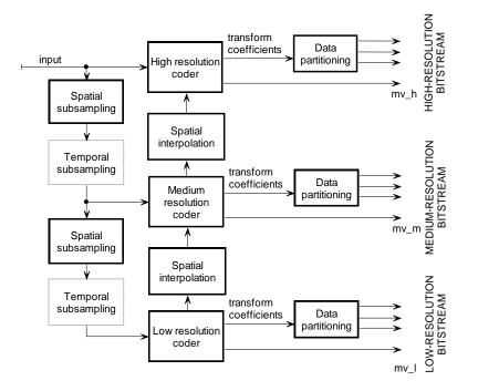
Fig. 2. A generic block diagram of the scalable coder as proposed in this paper.
