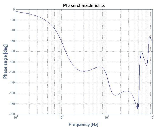
Fig. 7. Phase characteristics approximated using VF and weights, backward direction.
