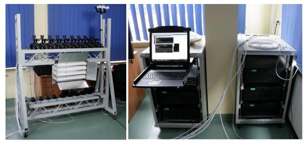
Fig. 6. Multi-camera rig (left) and recording system (right), both developed at Poznan University of Technology, Chair of Multimedia Telecommunications and Microelectronics, Poland.
