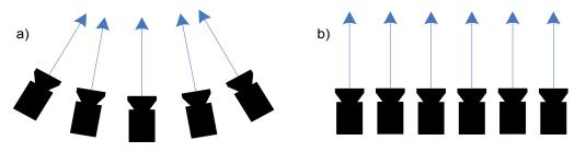
Fig. 12. Various arrangements of cameras: a) angular camera arrangement,b) linear arrangement of the cameras with parallel axesof the cameras (considered in the dissertation)
