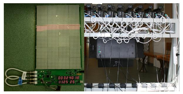
Fig. 7. Electronic board for multi-camera synchronization testing (left) and synchronization circuitry connected to the cameras (right), both developed at Poznan University of Technology, Chair of Multimedia Telecommunications and Microelectronics, Poland.
