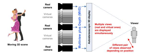
Fig. 2. Glasses-free 3D. Depicted "virtual cameras" are cameras that do not actually exist in the scene, but their content is synthesized basing on the content from existing ones.
