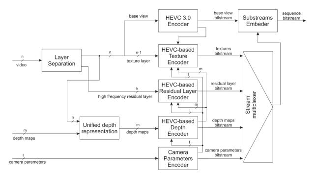
Fig. 76. The proposed 3D video encoder structure.
