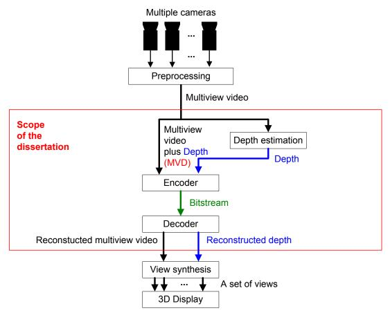
Fig. 4. The scope of the work (marked in red, dotted frame) as a part of the whole 3D video system.
