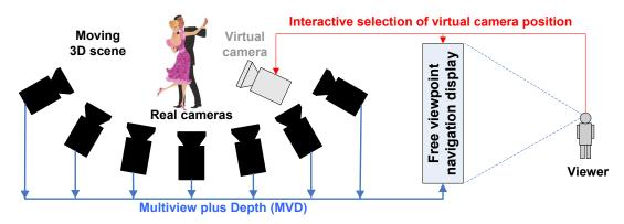
Fig. 1. Free-viewpoint navigation. Depicted "virtual camera" is a camera that does not actually exist in the scene but its content is synthesized from the content of existing ones.
