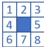
Figure 14: eight-pixel neighborhood for defining the connectivity criteria for region growing
