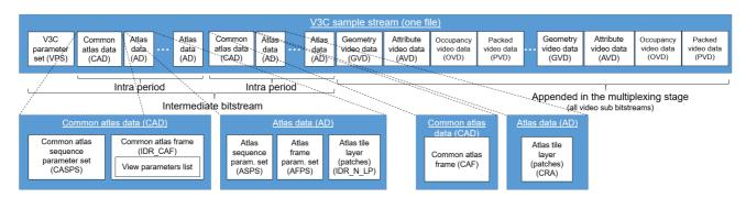
Figure 34: V3C sample stream with MIV extensions
