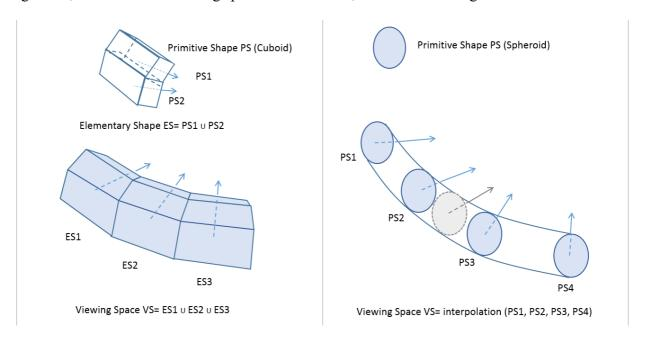
Figure 42: Illustration of VS creation with additive CSG (left) and interpolation (right)
