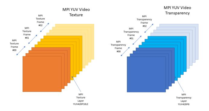
Figure 31: MPI raw storage diagram. In this simplified example, the MPI content is made of 4 layers (sorted from far to close) and 3 concatenated temporal frames
