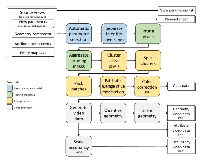
Figure 2: Top-level diagram of the TMIV single-group encoder
