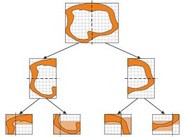
Figure 18: Recursive splitting of the cluster; dashed lines: C-splitting, dotted lines: L-splitting
