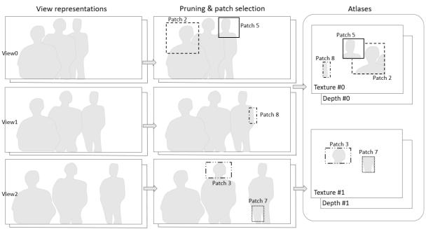
Figure 3: Representing source views using patch atlases
