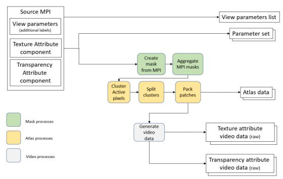
Figure 33: Top-level diagram of the TMIV MPI encoder
