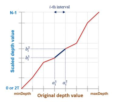
Figure 25: An example of piecewise linear scaling (for 7 intervals)
