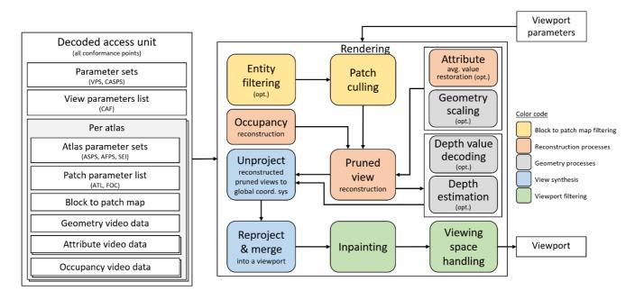
Figure 35: Process flow for the TMIV renderer
