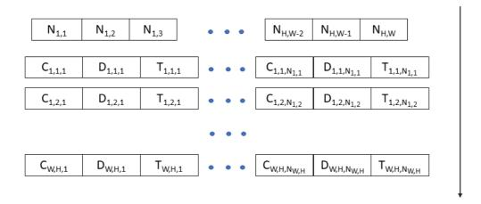
Figure 32: MPI packed compressed storage (PCS) layout.
