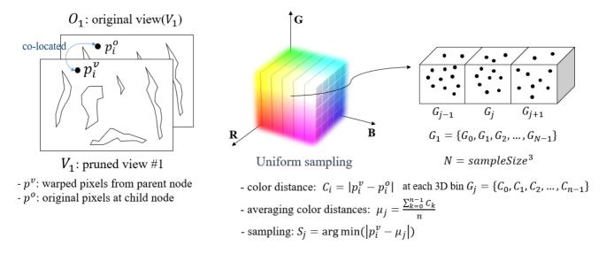
Figure 13: Uniform sampling in second-pass pruner
