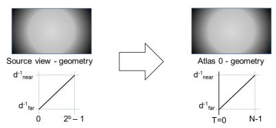
Figure 23: When the source material (with b bits per sample) has only valid geometry values, the geometry coder only performs u(b) to u(m) or u(m-1) scaling and the geometry threshold is set to zero to signal full occupancy;  $N = 2^m$  if the geometry has a good quality (§4.2.5) and  $2^{m-1}$  otherwise
