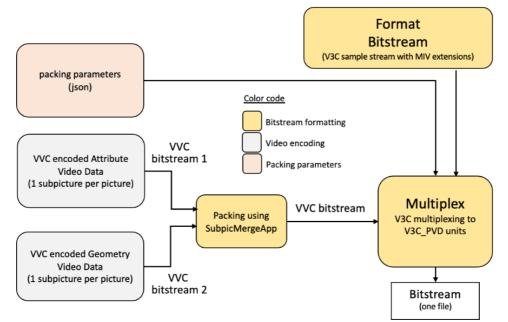
Figure 27: Encoding of texture and geometry components into one packed video sub-bitstream
