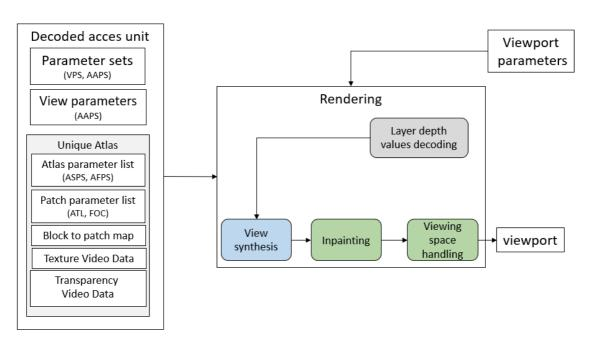
Figure 43: Process flow for TMIV MPI renderer
