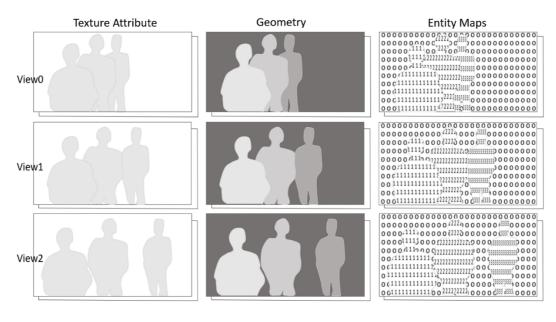
Figure 4: Input source views composed of texture attribute and geometry components, and entity maps
