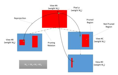
Figure 39: graph-based pruning: weight recovery procedure
