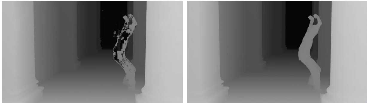
Figure 1: Coded depth of "Undo_Dancer" sequence with VSO turned on (left) and off (right).
