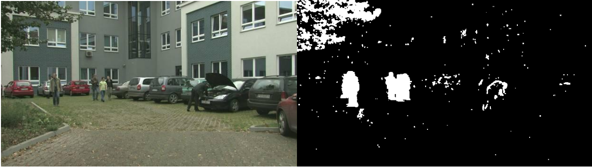
Figure 3. Motion map (right) obtained for exemplary frame (left) (white pixels – moving, black pixels – steady).
