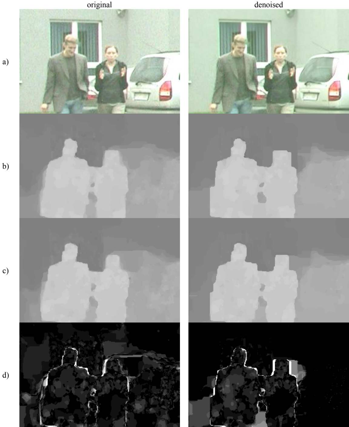
Figure 4. Exemplary results of proposed technique: original (left) and denoised (right). a) image b,c) depth maps for two consecutive frames d) difference between depth maps.
