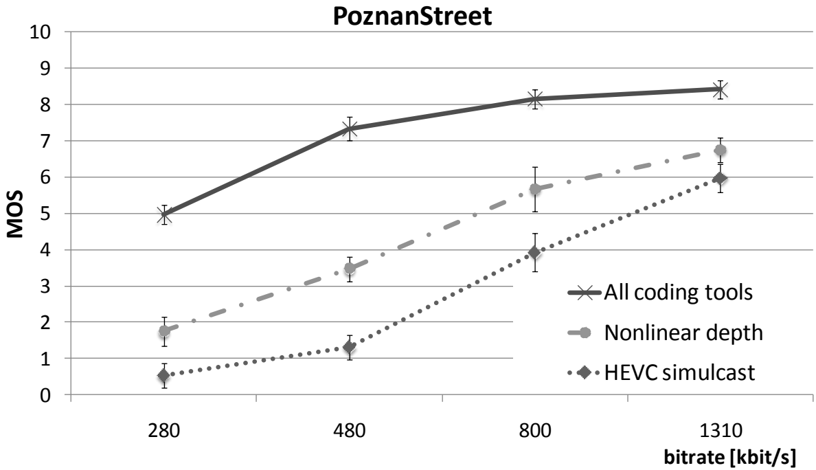
Fig. 6. Subjective test results for Poznan Street sequence.
