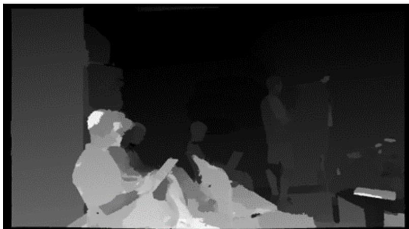
Depth map acquired by Kinect depth sensor:
