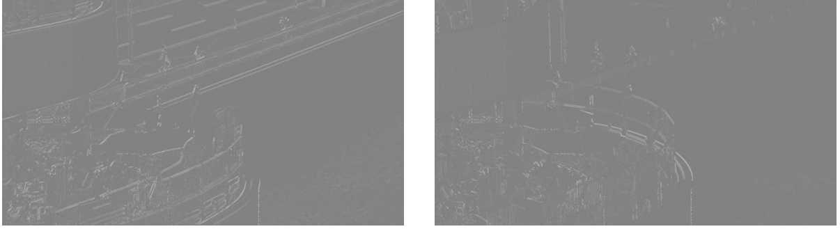
Fig. 1. The result of the 3x3 Sobel filter for 45-degree (left) and 135-degree (right) edges detection.
