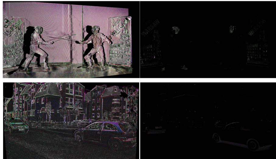
Figure 2. Comparison of the differences between the virtual view generated from the left view and the virtual view generated from the right view: Left column —original VSRS, right column —modified VSRS. From the top: Poznan Blocks, Poznan Street, Poznan Fencing 2, Poznan Carpark.
